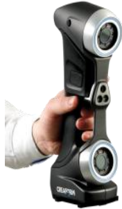
Fig 4: Handheld Laser Scanner
