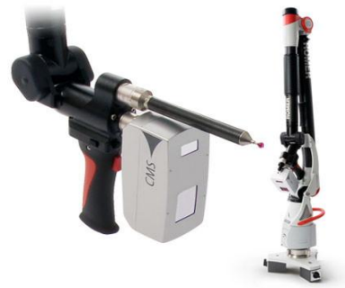
Fig 3: Articulating Arm Scanner
